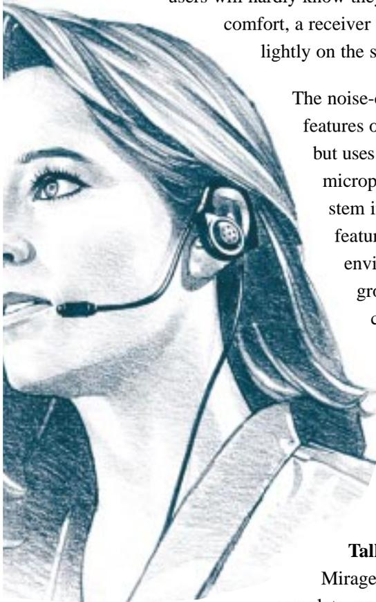
The noise-cancelling model has all the features of the standard Mirage headset, but uses a unidirectional noise-cancelling microphone mounted on a flexible stem in place of the voice tube. This feature is especially useful in busy environments where general background noise interferes with clear communications.
